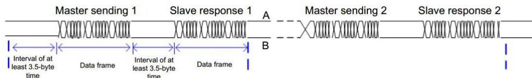
The communication protocol used by the drive is the Modbus-RTD slave communication protocol, which allows the drive to provide data to respond to "query/command" from the master or execute the action according to "query/command" from the master.
